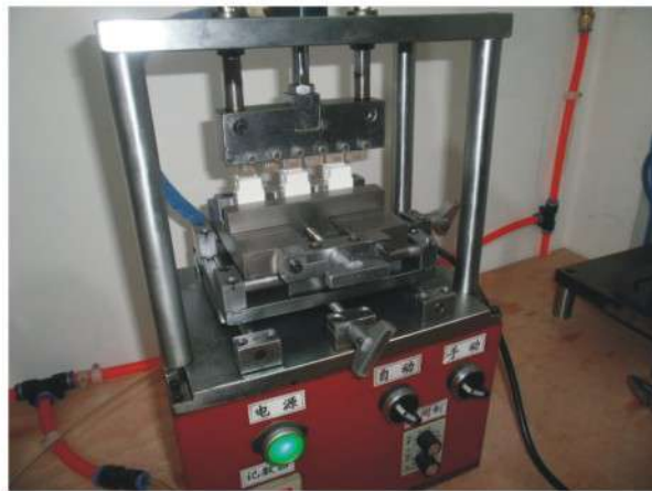
3 Auto-Tester of Insertion Life
